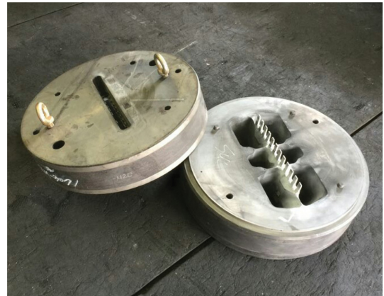
Fig. 10 Extrusion die for the overload detecting pad
