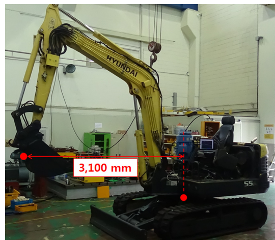
Fig. 6 A view of length of working device of excavator
