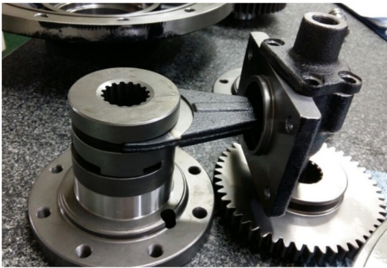
(a) Photo of a differential locking device
