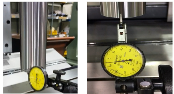
Fig. 10 Measurement environment of spindle run-out
