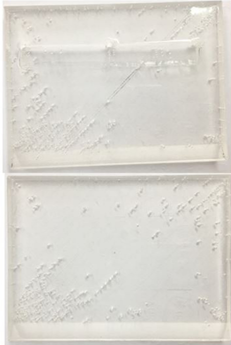
Fig. 9 Manufactured slot-die coater with PDMS
