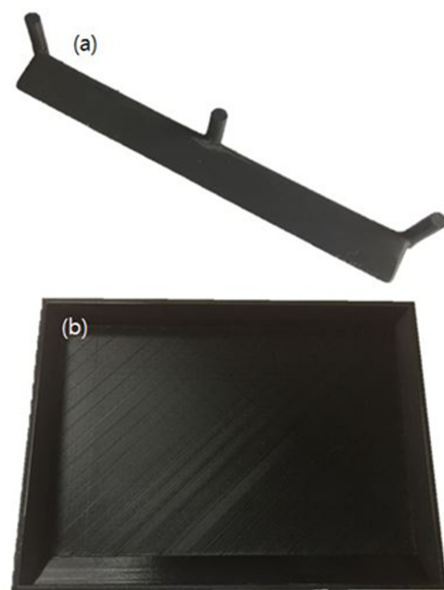
Fig. 7 Mold of slot-die coater: (a) Reservoir, (b) Coater mold
