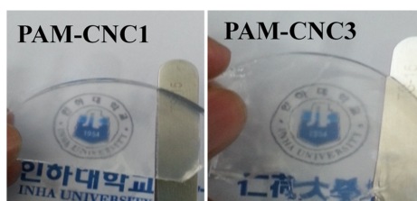
Fig. 5 Optical transparency of polyacrylamide and its composite hydrogel
