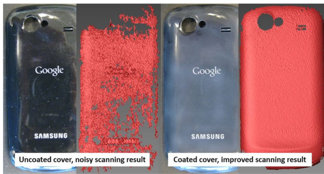
Fig. 7 3D scanning results of a shiny cell case
