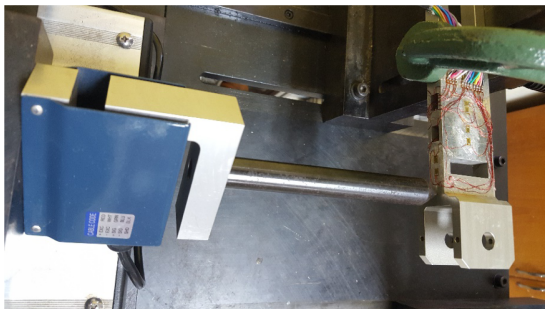
(b) Applied rated force Fx to three-axis force sensor
