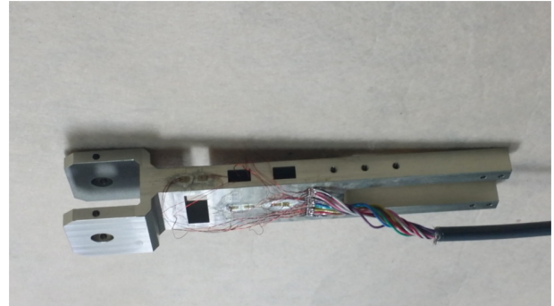
Fig. 7 Photograph of the manufactured thigh link three-axis force sensors
