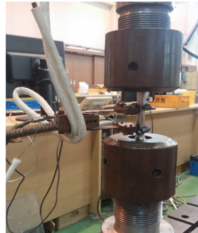
Fig. 2 Tensile test equipment and COD gauge
