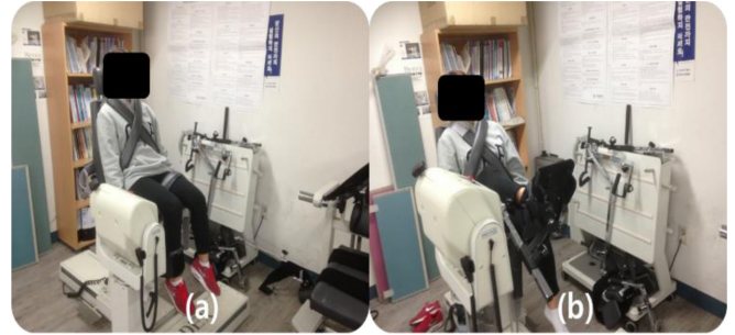
Fig. 1 Isokinetic joint torque test for estimating the muscle strength imbalance ((a): knee joint, (b): ankle joint)
