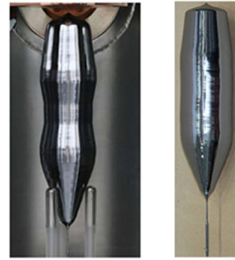
Fig. 2 The float-zone single crystals of highly 28 Si enriched silicon. These photographs are courtesy of the Leibniz institute for crystal growth (IKZ) 9
