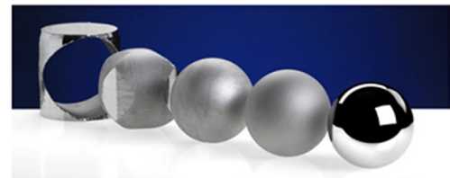
Fig. 3 Manufacturing of the highly 28 Si enriched silicon sphere 9
