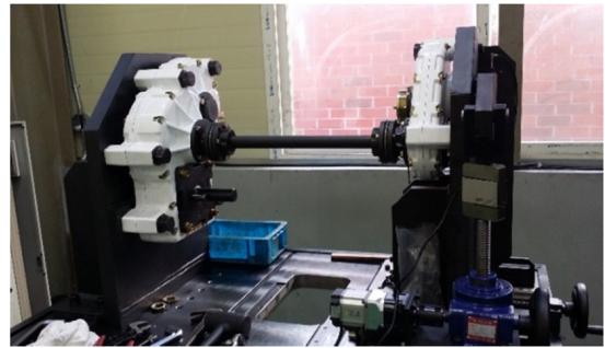
Fig. 15 Test bed shape of angle drive unit
