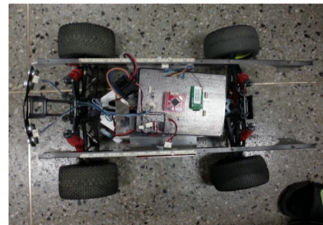
Fig. 15 Intelligent vehicle mounted with a camera
