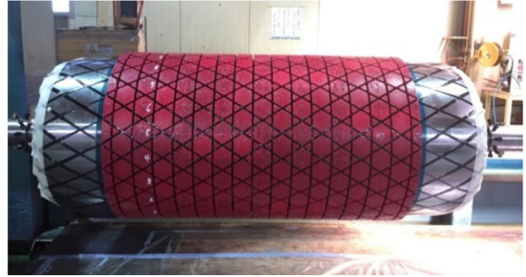
Fig. 1 Fiber winding process of cylindrical composite lattice structure
