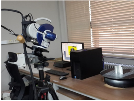
Fig. 5 Deformed shape measurement with 3D scanner
