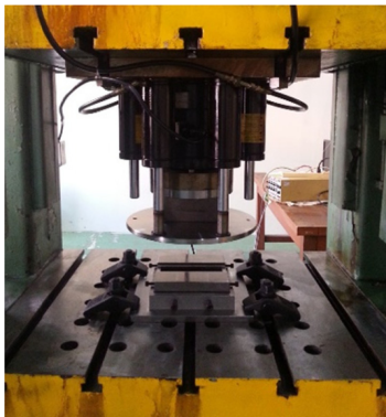
Fig. 3 Experimental setup for U-shape draw bending
