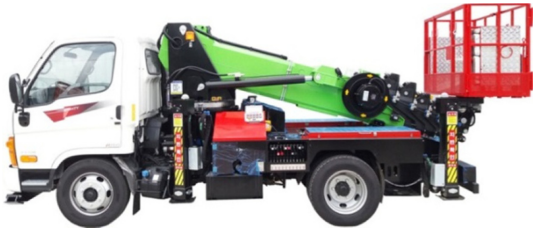
Fig. 1 Photo of aerial lift truck
