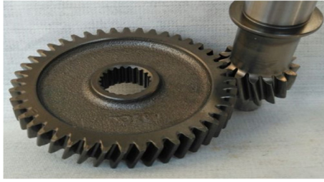
Fig. 4 The 1st helical gear pair
