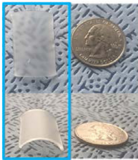
Fig. 6 Fabricated PDMS sensor body using aluminum mold
