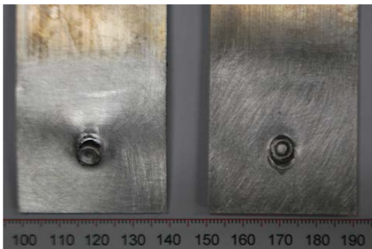
Fig. 6 Failure mode observed in the SPR joint specimen
