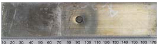
Fig. 2 Specimen configuration of SPR joint
