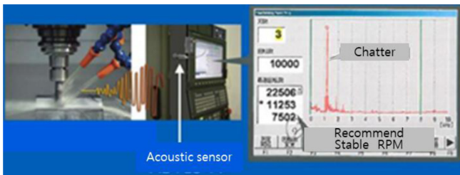
Fig. 17 Recommend spindle RPM with Machining-Navi
