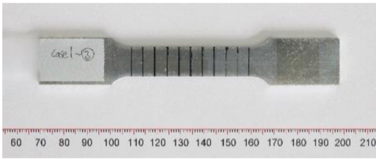
Fig. 1 Tensile test specimen (ASTM B557)
