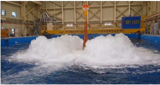
Fig. 3 Operation of vertical thrusters in URI-T
