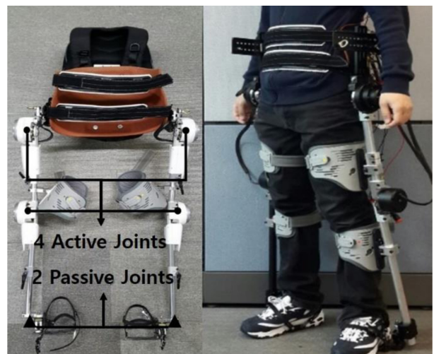
Fig. 1 WAP-2 (Walking assist robot for paraplegic patients ver. 2)
