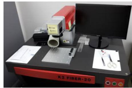
Fig. 1 1064 nm ytterbium pulsed fiber laser (Model: K2 Fiber 20, Manufacturer: K2 Laser System)
