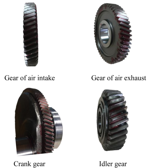
Fig. 9 Gear contact pattern of after mod. in bench testing
