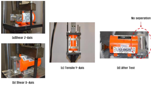
Fig. 7 Test and result of the shear and tensile test
