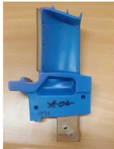
Fig. 1 Actual shape of 1st stage turbine blade
