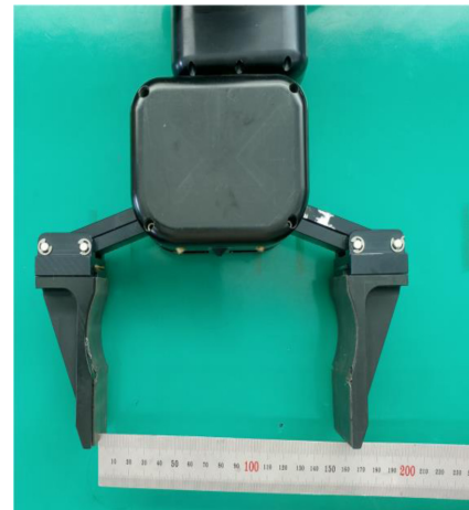
Fig. 13 Measurement of grip width
