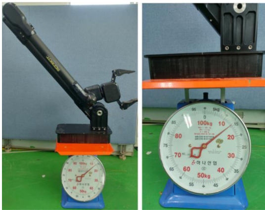
Fig. 10 Measurement of manipulator weight.
