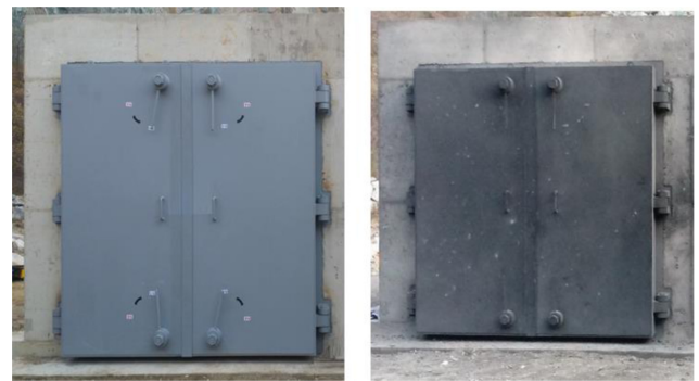
Fig. 3 Blast door used in explosion test
