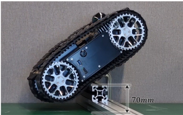
Fig. 8 Obstacle overcoming test of the developed robot
