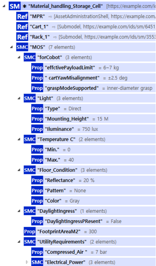
Fig. 3 AAS for material handling and storage cell control with emphasis on MOS
